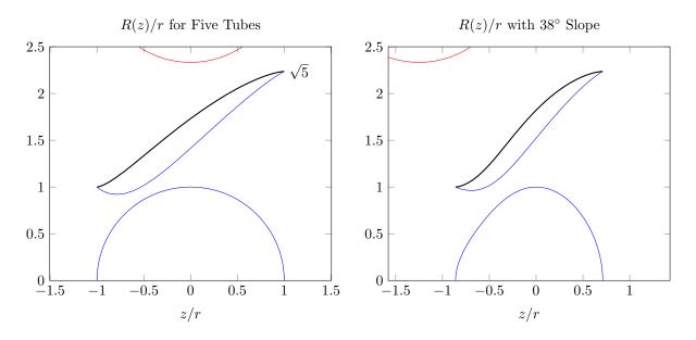
Using sloping tubes makes it easier to drain the unit and increases the minimum distance from the junction to the nearest tube of the other color. However sloping tubes add more fluid for a given value of z.
